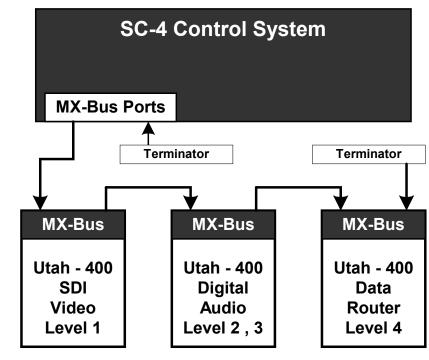
FIGURE 2-6. Block Diagram of an MX-Bus Daisy Chain
