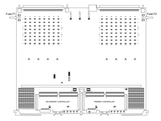
FIGURE 4-3. Main Board Fuse Locations
