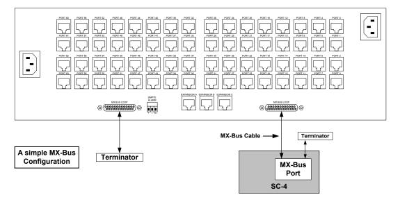
FIGURE 2-5. The MX-Bus Connection to an SC-4 Controller
