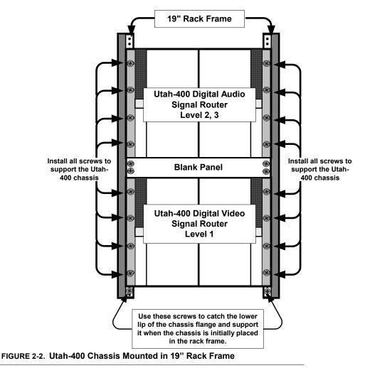
3. Install the Utah-400 chassis' in the 19" rack frame.
