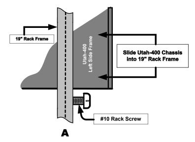
FIGURE 2-3. Sliding the Utah-400 Chassis into Rack Frame
