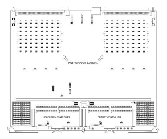
FIGURE 2-14. Main Board Assembly Port Termination Shunt Locations
