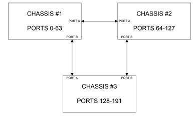
FIGURE 2-19. Utah-400 Data Router – 3-Chassis System
