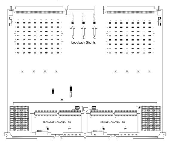
FIGURE 4-1. Loopback Shunts
