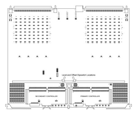
FIGURE 2-8. Main Board Assembly Dipswitch Locations
