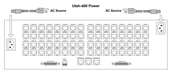
FIGURE 2-22. Utah-400 Data Router Power Connections
